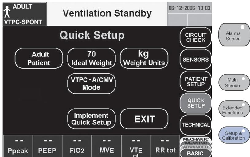
Figure F-9: Quick Setup Screen (Not available S model)
