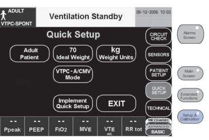
Figure F-9: Quick Setup Screen (Not available S model)
